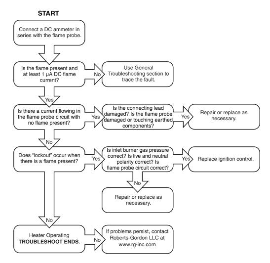
NOTE: Minimum flame probe current 1 µA DC. Typical flame probe current 3-5 µA DC.
